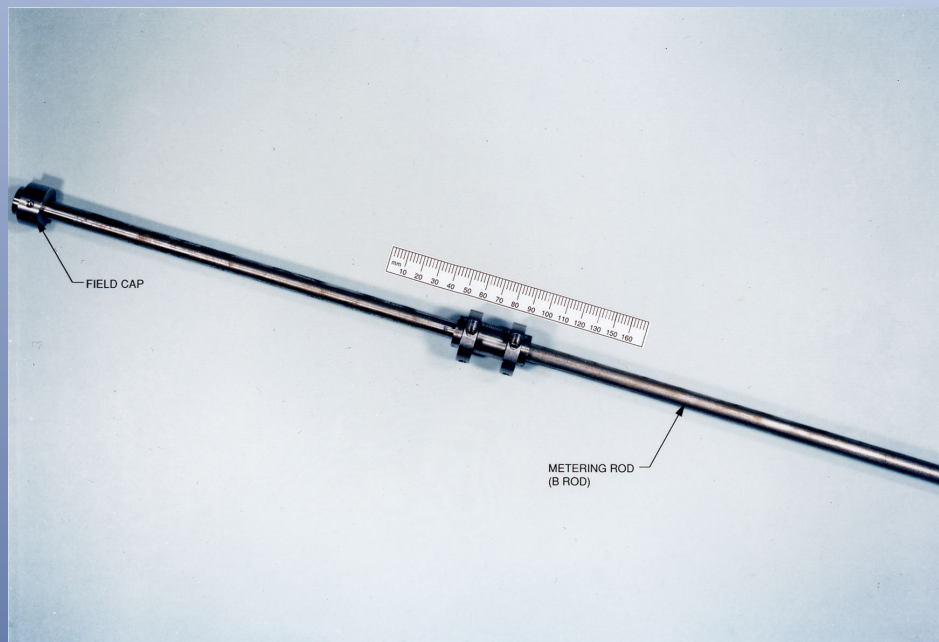
Figure 7-2. Metering rod (B rod) used to space the field lens and the center of curvature of the lower mirror in the reflective null corrector.
