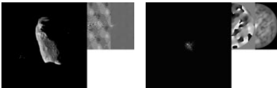
Figure 1. Simulated object on the left, and point-spread function that simulates aberrations by atmospheric turbulence of a ground-based telescope on the right (short exposure).
