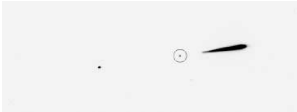
Figure 1: Sum of the direct image (F105W) and G102 exposure of the continuum source. The direct image is marked by a circle, and the grism +1st order can be seen extending towards the right. The grism 0th order is also visible as a point source to the left of the direct image.
