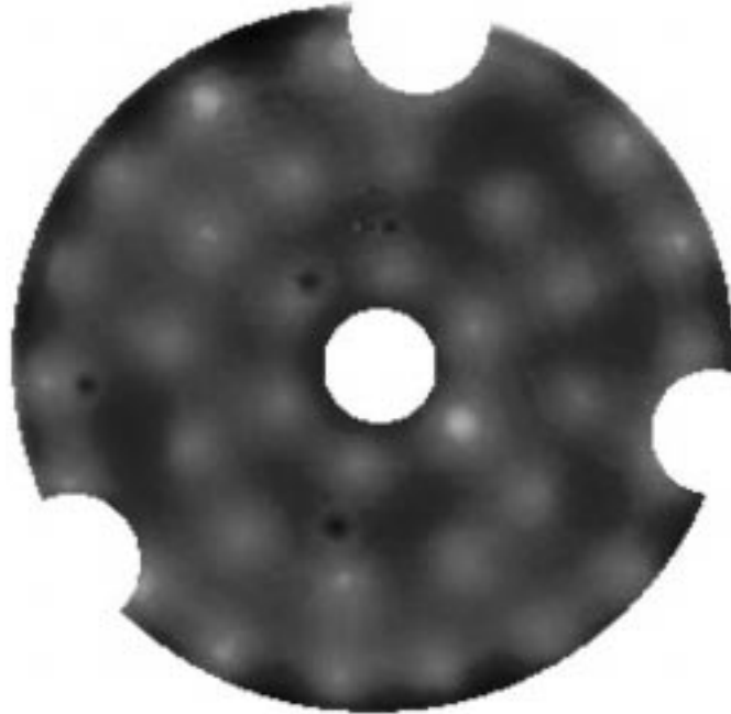
FIGURE 6.9. The Effects of Gravity on the Surface of the MARS. Laser interferometry reveals a small bump on the surface above each of the actuators. The measured departure from a perfectly spherical surface is 0.053 \mu\text{m} RMS. The calculated bumps for a 2 \mu\text{m} thick Zerodur shell is 0.050 \mu\text{m} RMS. (University of Arizona Mirror Lab, Composite Optics Inc.)
