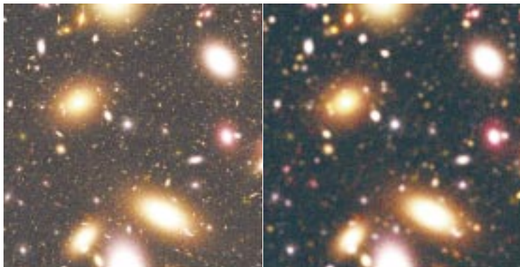
FIGURE 2.1. A comparison of a simulated NGST image with 0.06" resolution (left side) at the K band and one with 0.25" resolution (right side). Note that many of the faint galaxies are lost in the latter image because of confusion and lower sensitivity (ST ScI).
