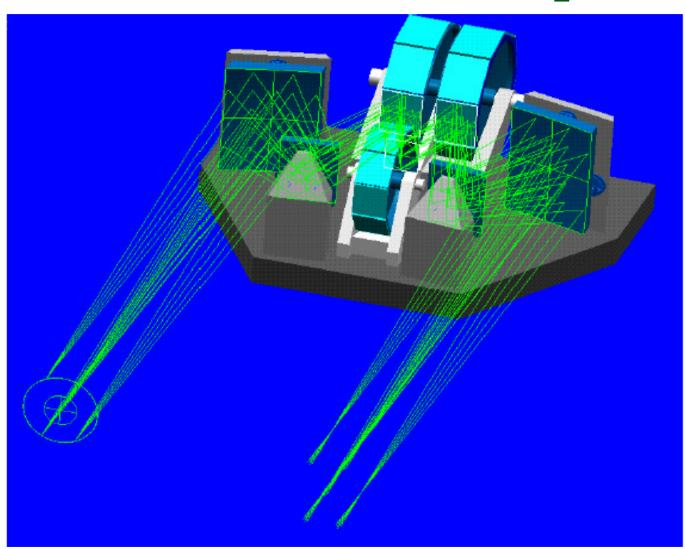
0.6-5 μm 3 x 6 arcmin FOV 0.03 arcsec/pixel
